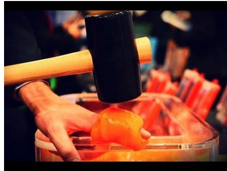
Figure 9: D30 Material Protecting Hand from Hammer
